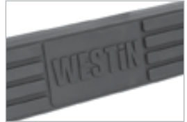
MOLDED POLYMER STEP PAD REPLACEMENT PART NO. 23-0001
