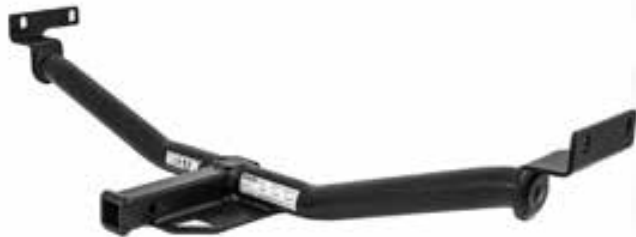
CLASS I — 2,000 LB TOWING CAPACITY
